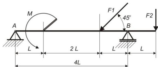
$$M=7 \text{ kNm}, F_1=3\sqrt{2} \text{ kN}, F_2=2 \text{ kN}$$
